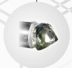
Sticking on Sawing Bit
