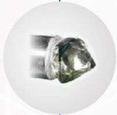
Sticking on Sawing Bit
